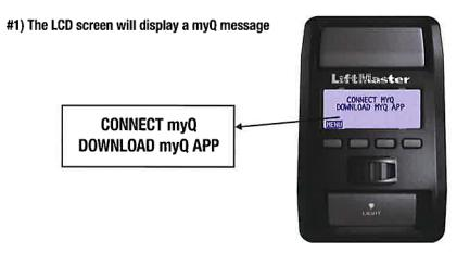
The message will display for 10 seconds every time the door opens or closes and then will go back to the time/temperature screen. The message will stop displaying when:
