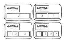
Set Switches 1 through 9 at any security code, press and hold desired channel. Now press learn. The green LED will flash indicating the channel is stored. One flash is for channel one, two for channel two, three for channel three, and four for channel four. The transmitter has now stored the code in the coresponding channel until the learn switch is pressed again.
