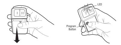
Press and release the button. When the LED stops flashing, continue to press and release the button until a click is heard from the garage door opener, a light on the garage door opener blinks, the garage door opens/closes, or a beep is heard from the gate operator (maximum 18 times).
