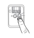
**1.2** Press and hold the UP Button until the door is in the desired UP position.
