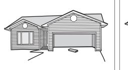
**2.2** Press the remote control push button to close the door. The door MUST reverse when it makes contact with the board.
