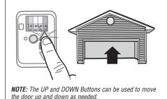
**1.3** Once the door is in the desired UP position press and release the Adjustment Button. The garage door opener lights will flash twice and the DOWN Button will begin to flash.
