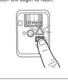
1.6 Press and release the UP Button. When the door travels to the programmed UP position, the DOWN Button will begin to flash.
