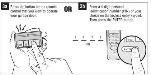
The garage door opener lights will flash (or two clicks will be heard) when the code has been programmed. Repeat the steps above for programming additional remote controls or keyless entry devices.
