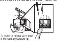
**PRE-WIRED INSTALLATIONS:** Connect the same wires to the garage door opener that were previously connected to the door control.
