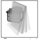
The sensor must not have any object likely to move or vibrate in its sensing field.
