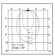
The sensing fields here on the right correspond to the following adjustments: • tilt angle: 15°, 30°, 45°;
