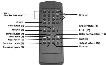
**Remark:** For optimum results point the remote control at the sensor before pressing its buttons.
