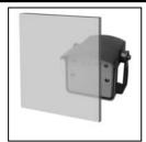
The sensor must not be placed directly behind a panel or any kind of material.
