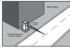
To comply with UL325, installation of secondary entrapment protection devices is required with this operator. Ask your installer which safety device is correct for your application.
