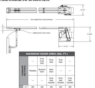
NOTE: On steel insulated doors, a 24-gauge back panel is assumed. If a heavier back panel is supplied, use the next higher HP rating. Recommended Duty Cycles: 25 per hour, in excess of 90 per day.
