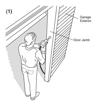
**Step 2:** (Illustration 2). If your garage has a built-up jamb, drill the hole to a depth of 2" (5 cm). Then on the inside jamb, drill a second hole into the first hole to complete access.
