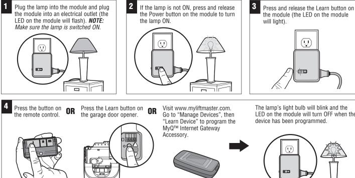
The lamp's light bulb will blink and the LED on the module will turn OFF when the
