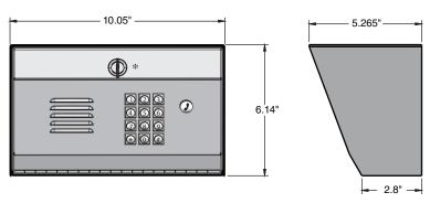
Power Supply: 12 Vac 20 VA or 16 Vdc 2.5A
