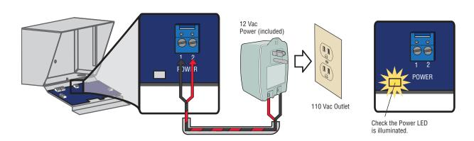
**NOTE:** Once power is applied, the EL1SS will begin to **click** to indicate that it is powered, and is waiting to be programmed for the unit's Master Code. The Master Code is used to unlock the programming functions of the EL1SS. The Master Code should not be distributed as a User Code.
