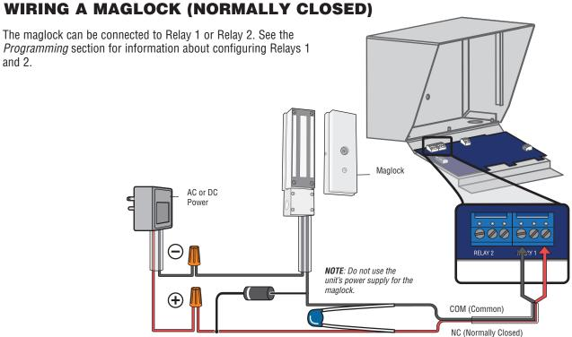
**NOTE**: For DC power install a 1N4001 diode or equivalent.
