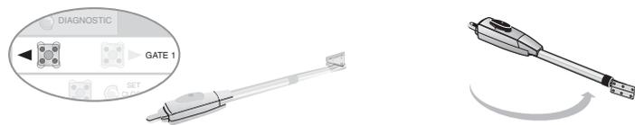
Press the **GATE 2** left button to move the left operator into the OPEN position.
