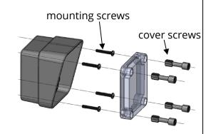
**8.** <u>SECURE COVERS:</u> Using the provided plastic screws secure the cover snug (don't overtighten them).
