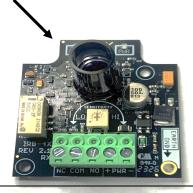
**6.** <u>TEST OBSTRUCTION:</u> Place an obstruction (such as your hand) between the TX and RX and the RX's OBS LED should TURN ON when obstructed (and turn off when not obstructed and aligned). Test at different distances.
